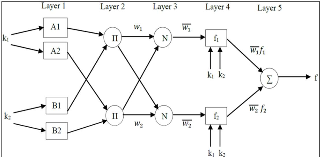
Fig. 2: The adaptive neuro-fuzzy inference system architecture
