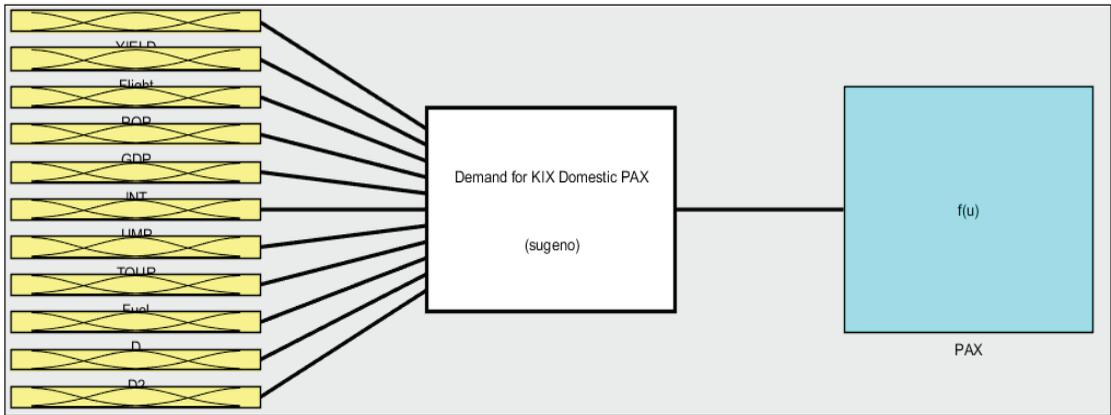
**Fig. 3:** The structure of Kansai International Airport domestic airline passenger ANFIS forecasting system
