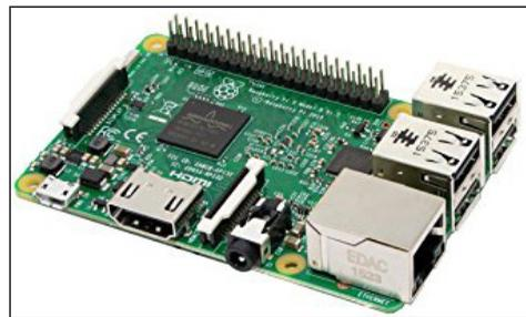
**Fig. 2:** Raspberry Pi Development Board
