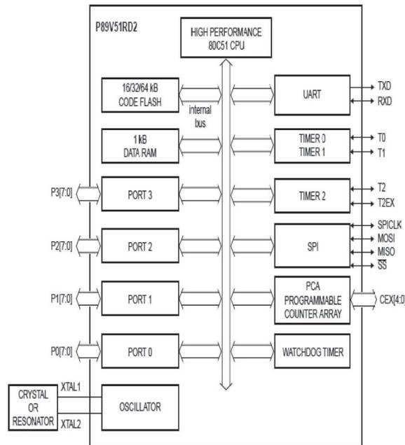
Figure 3: Block diagram of P89V51RD2 microcontroller.
