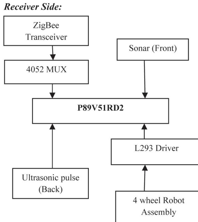
**Figure 1:** Block diagram of accelerometer based robot motion and speed control with obstacle detection
