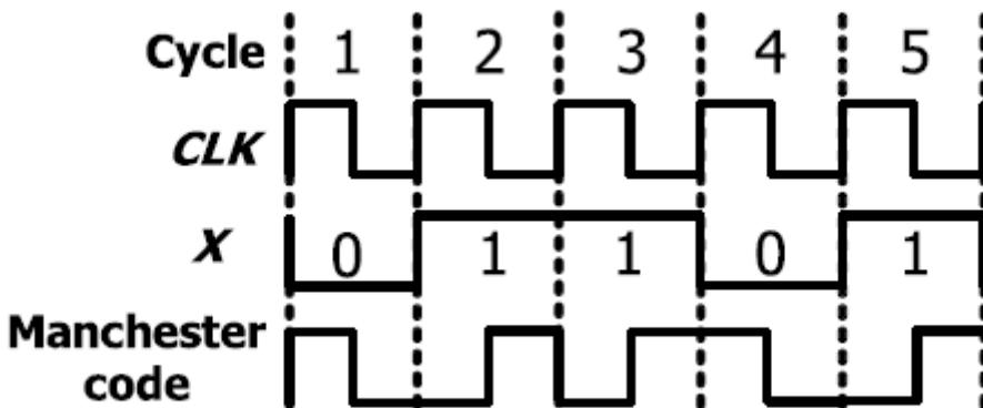
Figure 3. Illustration of Manchester coding example.
